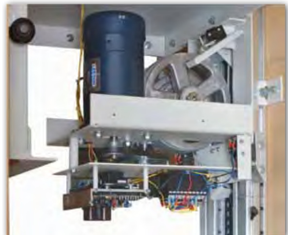
Electric motor, cable-drum drive system and limit switches are pre-installed under the car.
